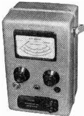
Valve milli-voltmeter Type TF899 made by Marconi Instruments.
